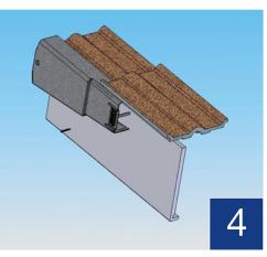
Fix the top edge of the Verge Cap to the barge board using a Spacer Tube and screw. Spacer Tubes are easily cut to length using shears.
