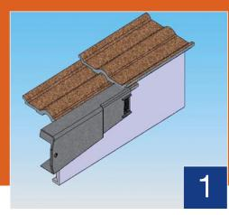
Starting at the bottom, slide the top leading edge of the Verge Cap under the bottom edge of the second row of tiles.
