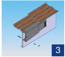
After completion of stages 1 & 2, the lip at the bottom end of the Verge Cap should be in contact with the bottom edge of the tile. Fix the lower edge of the Verge Cap where convenient, using a Spacer Tube and screw and finish by inserting the Screw Cover Cap.
