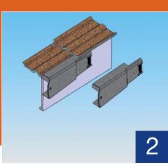
If the tile is securely fixed with cement, preventing installation, notch the Verge Cap as required. This is easily achieved with the use of shears.
