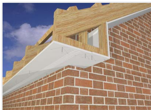
Fig 9. Typical GPB soffit installation.
