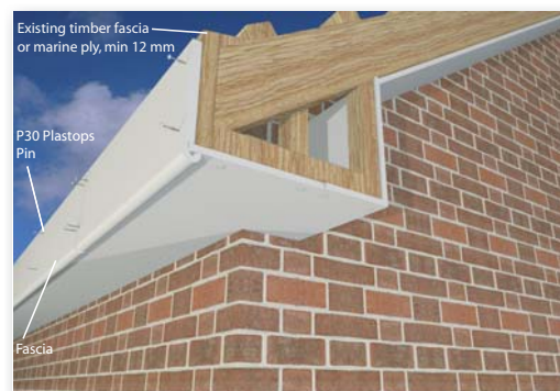
Fig. 17. Standard over-fascia installation.
